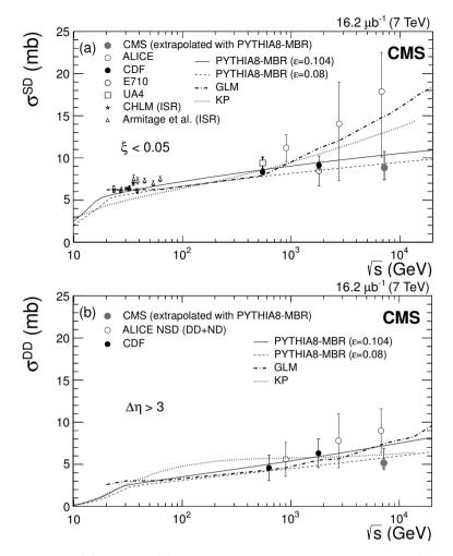
Fig. 1. Measured (a) SD and (b) DD cross sections for forward proton/antiproton momentum loss  $\xi < 0.05$  compared with theoretical predictions. The PYTHIA8-MBR model describes well all the measurements (from Ref. [10]).
