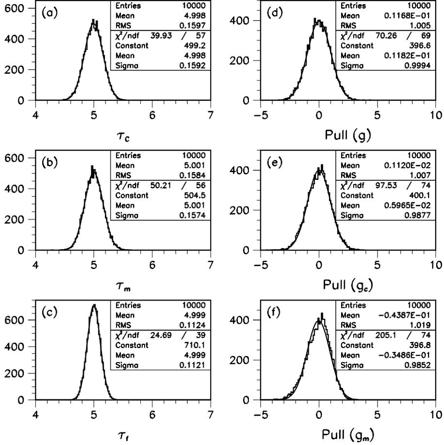
Figure 5: Results of a pseudo-experiment run with  $\tau_g = \bar{\tau}_c = 5$ ,  $\sigma_c = 0.1581$  and  $N = 1000$  (see text). Plots (a), (b) and (c) show distributions of the constraint  $\tau_c$ , the unconstrained fit result  $\tau_m$ , and the constrained fit result  $\tau_f$ , respectively. Plots (d), (e) and (f) show pull distributions according to definitions (27), (10) and (11), respectively.
